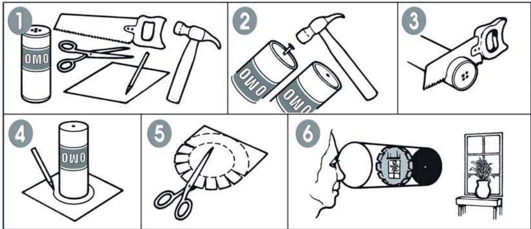
Figure 7.2 Home-made camera obscura. (Paint its inside surface matt black for best results.)
